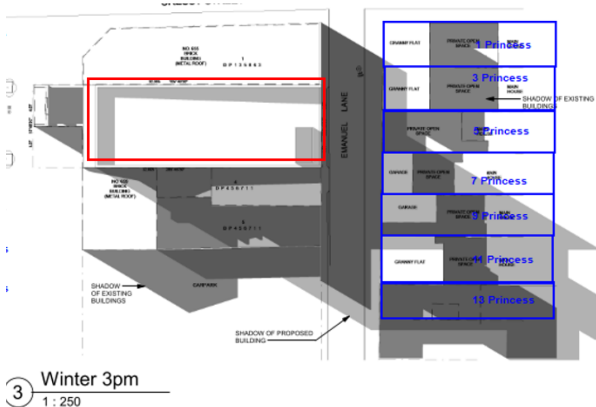
Figure 13: Shadow Diagrams June 21 at 9am, 12pm, and 3pm and location of affected properties (blue) and subject site (red).
